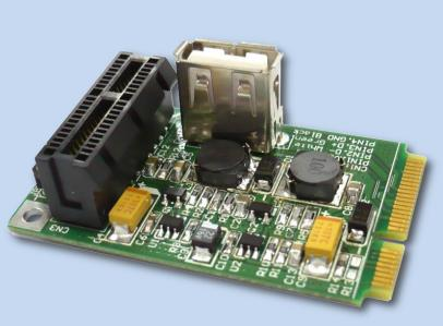
The PCI-E 1x to Mini PCI-E Card 1.0 is a debug tool for PCI-E interface card. This module allows you to use your existing PCI-Express Add-in-Card in the Mini PCI-E slot.
