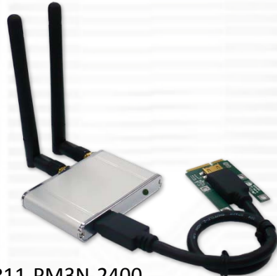
MR11-PM3N-2400 with ANT2400Q2P3 x 2pcs (2.4GHz 2.15dBi Rubber duck antenna)
