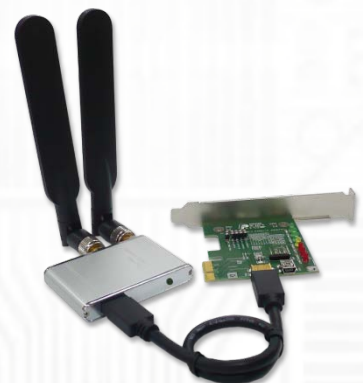
MR11-HP1A-2458 with ANT2458Q5P x 2pcs (2.4/5.8GHz Rubber Duck Antenna)
