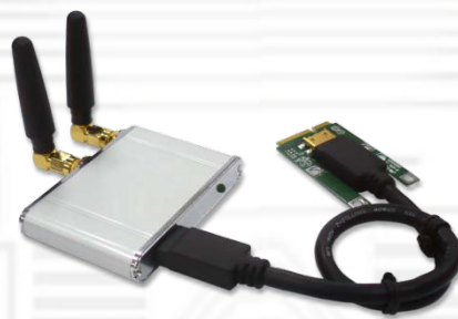
MR11-PM3N-0918 with ANT0918Q2P1 x 2pcs (900/1800MHz 2dBi Portable Antenna)
