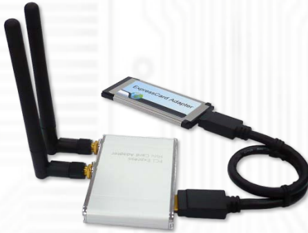
MR11-EC2C-2400 with ANT2400Q2P3 x 2pcs (2.4GHz 2.15dBi Rubber duck antenna)
