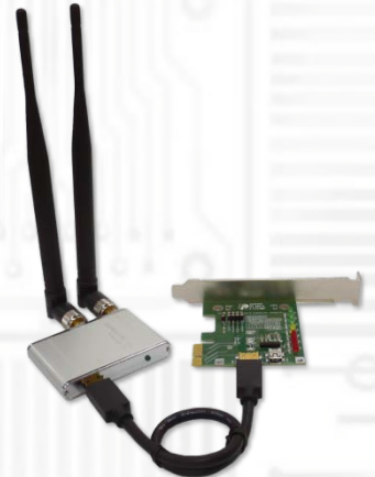
MR11-HP1A-5800 with ANT5800Q5P x 2pcs (5.8GHz 5dBi Rubber Duck Antenna)
