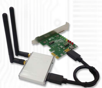
MR11-HP1A-2400 with ANT2400Q2P3 x 2pcs (2.4GHz 2.15dBi Rubber duck antenna)
